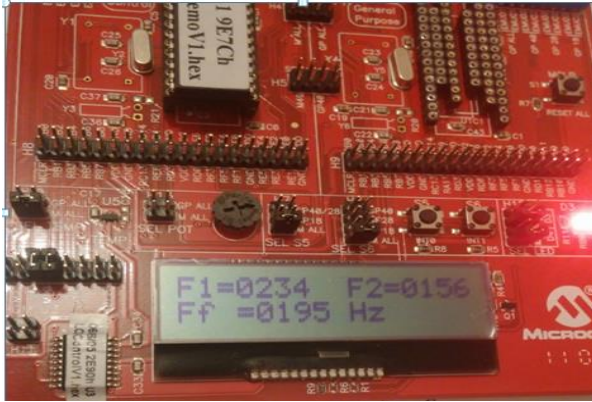
Figure 24: Frequencies display as an output of the DSPICDEM card
